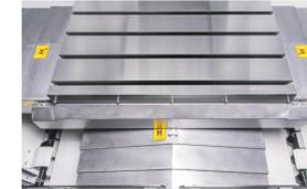
**SLOPE ON TELESCOPIC COVER FOR EASY CHIP FLOW**
