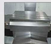
▲ 伸縮防屑蓋斜度設計 Slope on telescopic cover for easy chip flow
