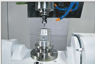
▲ V100 (4+1軸) 4+1 Axis 4+1 定位加工 4+1 Position cutting
