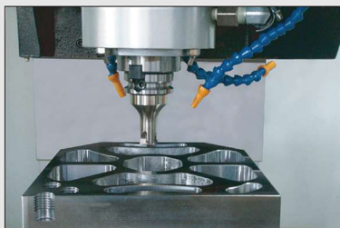
▲ V100 粗銑挖槽加工 Wide milling cutting
