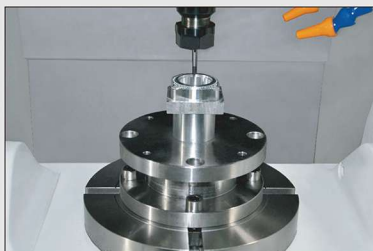
▲ HV70 (4+1軸) 4+1 Axis 4+1 軸錶殼加工 (AL7075) 4+1 Watch bezel cutting
