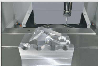
▲ HV70 雕銑加工 (AL7075) Milling & engraving cutting
