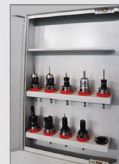
▲ 增加刀倉設計 Second tool magazine located in front of the machine
